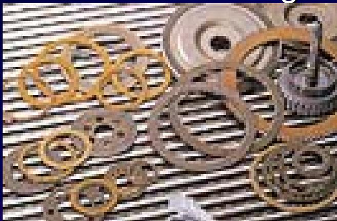
Automobile-use wet-type friction material made of high-performance paper (more than ten layers)
